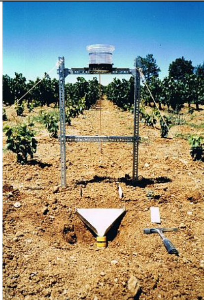
A rainfall simulator was used to determine the infiltration capacity of the soil.
